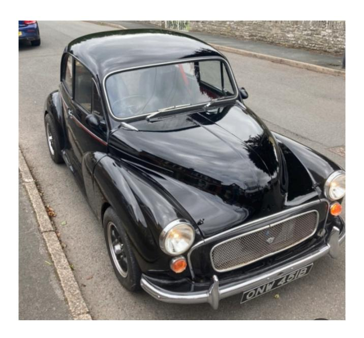
Wilma: 1964 Saloon, extensively modified to include a Rover V8 engine with space cage and all usual upgrades to suspension, brakes, greabox etc to make the RV8 safe and usable. Is currently 'as-acquired' but will be a project for me to bring fully up to scratch.
