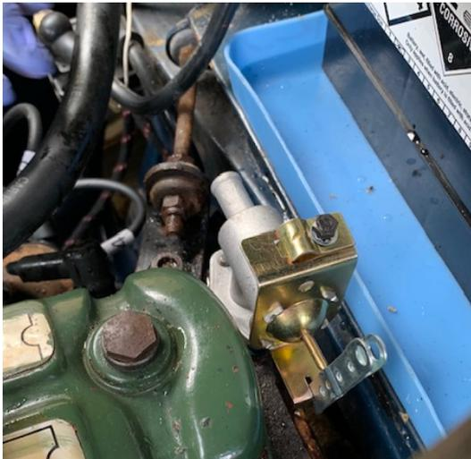
6. Nuts finally on and a pleasure to refit the hose - after freshening up the end by removing a couple of centimetres.
